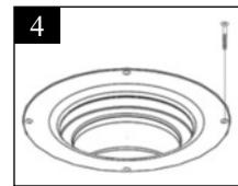
4 Pilot section (4) and screw down using 3.0 x 20mm (No.4 x 3/4") screws. Do not use power tools.
