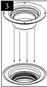
3 Push gully section (4) firmly inside the middle section (5) until they click together
