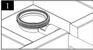
1 Measure Maxxus drain location and then Connect section (7) of the gully securely to waste pipe using solvent-weld adhesive centrally underneath the hole of the tray.
